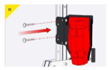
Insert the retaining pins to secure in place on the Upright
