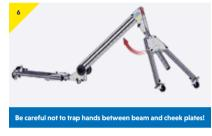
Scissor upper A-Frame until ball-lock pin is adjacent to beam
