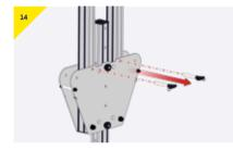
While in this vertical position remove ball lock pin from its stow hole
