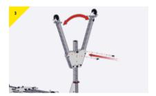
Open leg and insert ball-lock pin into second hole securing the leg in its open position. Repeat for second leg on the same A-Frame.
