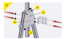
> Present bracket to gantry as shown (with locating pin at bottom) and insert new, longer bolts securing the winch with the quick release knobs provided
