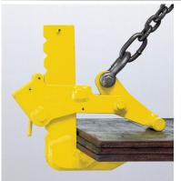
\*Chain slings and shackle NOT included **The ACH horizontal plate clamps** offer superb flexibility because of the large adjustable jaw opening. The jaw is adjusted using a simple ratchet mechanism.
