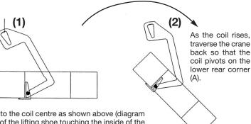
Place the hook into the coil centre as shown above (diagram 1), with the back of the lifting shoe touching the inside of the coil and the lifting sling vertical. Slowly hoist up until the coil rises from the ground.
