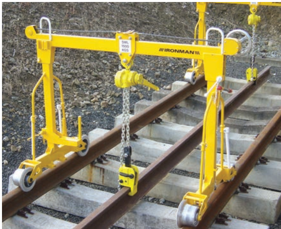
Typical application shot showing a CR1000 in use with a Yale D85 Pul-lift and an 'Iron man'.
