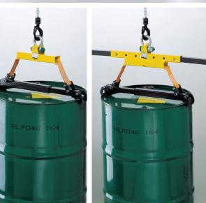
The DA drum grab is designed for the vertical transportation of steel drums. The jaws grab under the lip of the drum with its form-fitting connection.
