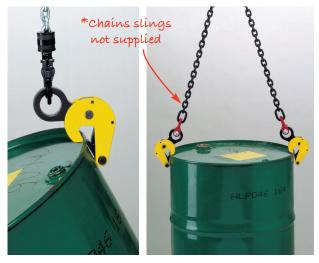
The DC500 drum clamp has been designed to lift and transport steel drums. If moving empty or sealed drums then one clamp is sufficient. Should you be lifting an open full drum, then two clamps should be used with a two leg chain sling.
