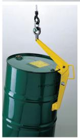
The DCV500 drum clamp has been designed to lift and transport steel drums in the vertical position. One clamp can be used to lift drums with or without their lids by gripping the rim of the drum.
