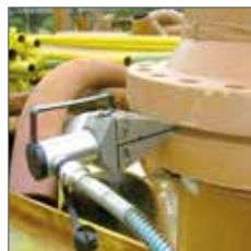
Spreading wedges YSW-14T 14t
