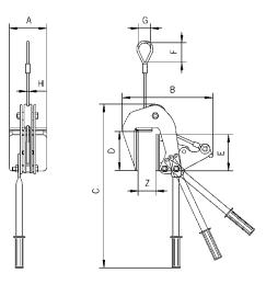
TPZ, up to 400 kg equipped with rope, from 750 kg equipped with chain.
