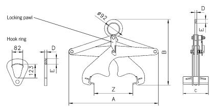
Hook ring for grabs for 2000 kg and above. Locking pawl keeps the grab in the open position.
